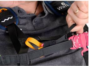
asymmetric collapse of the sail. There is also a second strap which lets you adjust the distance between the shoulders which, in case you forget to fasten the chest, prevents the pilot from falling out.
