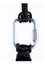
The two connections should be made using screw-lock karabiners with a breaking strength of at least 1,400 kg. In any case, it is important to verify that the length of the bridle is sufficient to position the reserve parachute inside the harness pocket, and that there is sufficient play to enable the parachute to be taken out of the pocket without causing the reserve parachute deployment bag itself to open during extraction.
